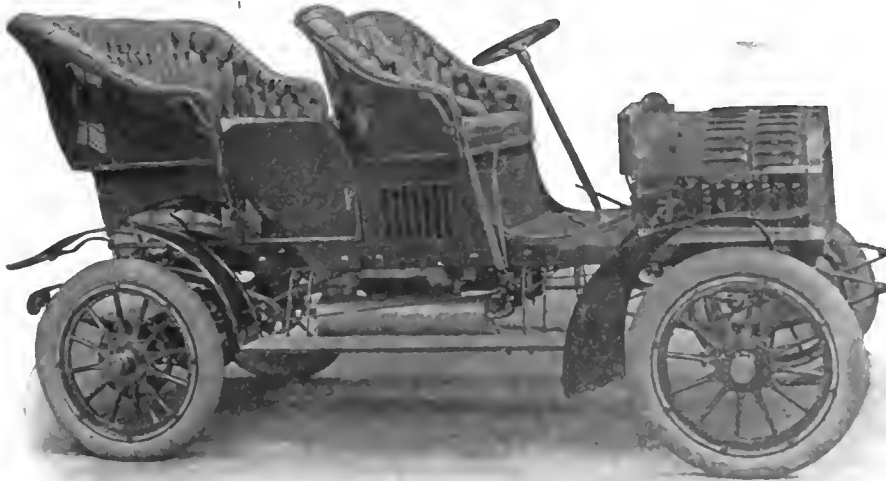
RELiance TOURING CAR. WITH DOUBLE OPPOSED MOTOR, SHOWING SIDE ENTRANCE.
